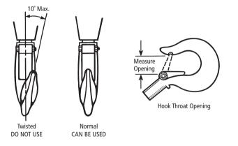
Any hook that is twisted or has excessive throat opening, indicates abuse or over loading of the unit. Other load sustaining components of the chain block should be inspected for damage. The chart above should be used to determine when the hook must be replaced. To measure throat opening, depress the latch against the hook body as shown above.
