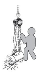
**DO NOT** shock load chain block, chain or hook.
