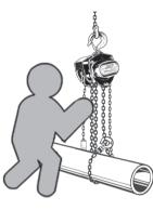
**DO NOT** wrap the load chain around the load and hook onto itself as a choker chain or bring the load in contact with the chain block.
